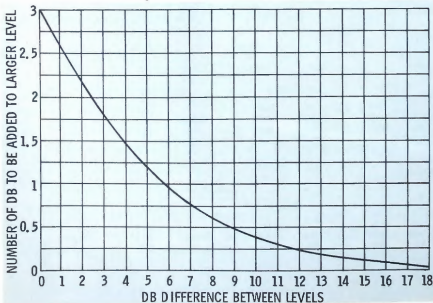
Fig. 1. Graph shows the result when two different noise levels are combined.
