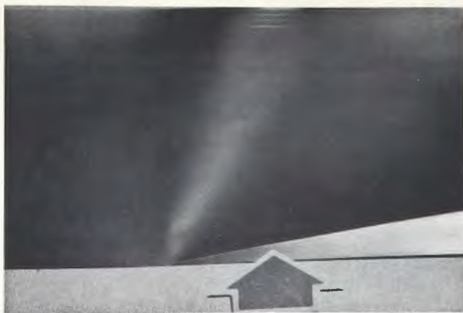
Fig. 7. Creases cause oxide buildup, high tip-wear rates.
