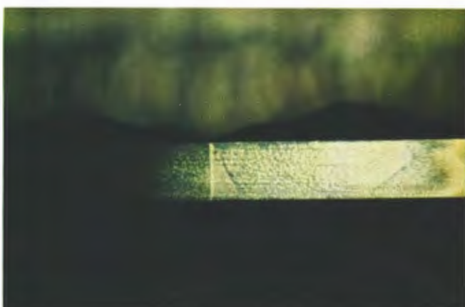
Fig. 4. Head tips exhibit blue-green and brown color. Coloration increases in density over 80 to 95% of the tip area. (Note appearance of Alfesil grain structure.)
