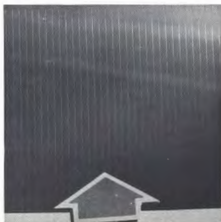
Fig. 10. Transverse burns from passing over a damaged tape cause wear.
