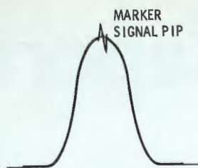
Fig. 3. Bandpass curve showing a marker pip to indicate center of passband.
